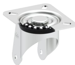
V-Type Ball Protector to prevent dust manifestation and maintain steel balls' position (NBLJ Type)
